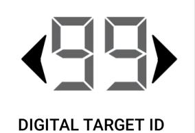
Numeric identification scale from 0 to 99. Identifies a target metal's conductivity.
